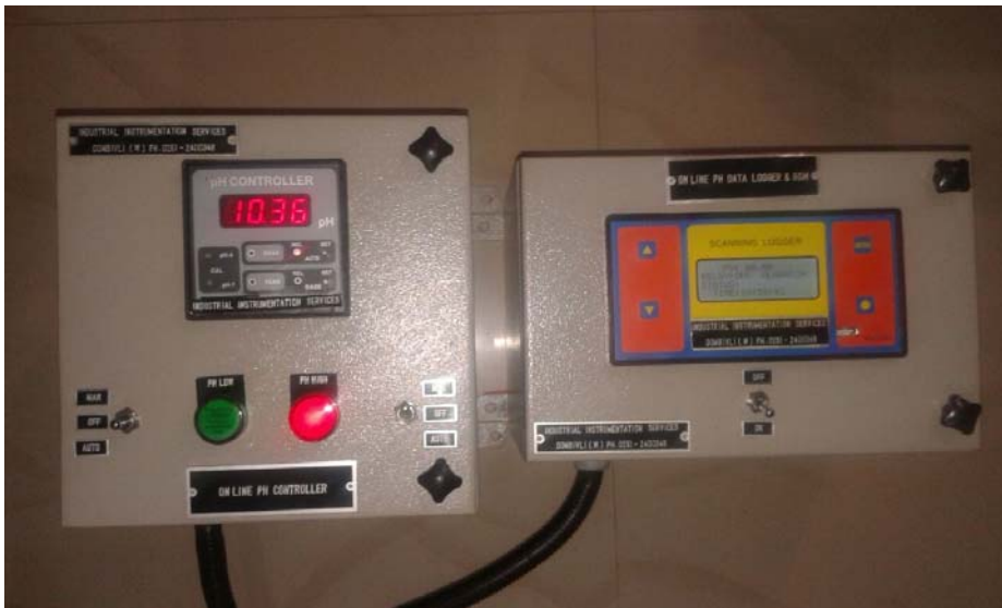
PH INDICATING CONTROLLER-TRANSMITTER-DATA LOGGER & GSM MODEM FOR SMS ALERT
