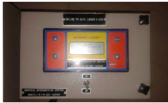
PH INDICATING DATA LOGGER & GSM MODEM FOR SMS ALERT
